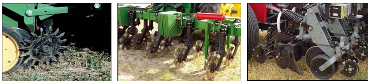
Figure 1. Examples of strip-tillage tool categories. (Left to right: Row cleaner, shallow strip-tillage tool, deep strip-tillage tool).
